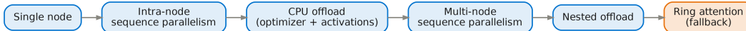
Figure 6: Memory-scaling ladder used during development. As context length increased, training progressively escalated from a single-node configuration to sequence parallelism, CPU offloading, multi-node sequence parallelism, nested offloading, and finally Ring Attention. Most experiments were run on the lowest rung capable of supporting the target context length, minimizing system complexity while preserving rapid iteration.
